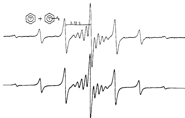
Figure 1. ESR spectra (upper) of a mixture of [benzene]/[benzene- d_6 ] = 0.36/1 reduced with a very deficient amount of potassium metal in THF and recorded at -100^\circ\text{C} . The computer simulation (lower) is based upon an anion radical ratio of [\text{BZ}^{\cdot-}]/[\text{Bz-}d_6^{\cdot-}] = 1.33/1 .
